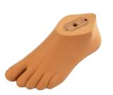
The 1K10 is a robust dynamic foot with a natural shape, smooth surface, and fully shaped toes. The foot features a contoured core and employs foams with a variety of characteristics. As a result, it offers a pleasant heel strike as well as easier roll-off and better energy return than the SACH\* Foot. The 1K10 is designed for use with modular or exoskeletal prostheses and can be combined with a modular adapter or shaped ankle part.
